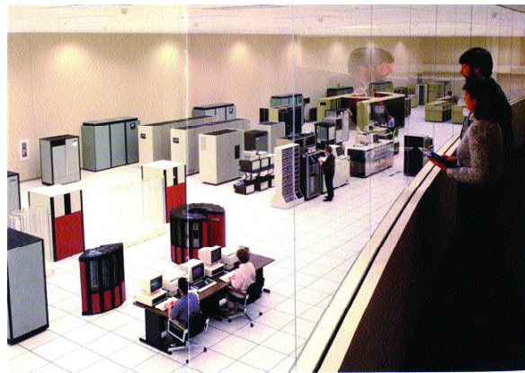
Figure 1. MSC computer room with prototype and production Cray 2s and a Cyber 205.
